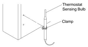
Figure 5 - Attaching Thermostat Sensing Bulb
